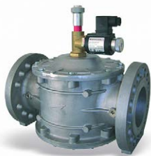
Electroválvula de gas rearme manual n.c. Pmax: 6 bar mod. EV125/6b 230VAC bridas DN-125 GIULIANI ANELLO
