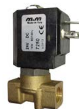
Electrovalvula Mm N.C 1/4" 24v Cc 0-16 Bar Diam 4 Mm Mod.D263dv17250
