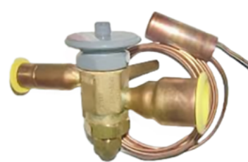
Valvula termostatica SPORLAN ERZE-12- 1/2, 5/8' x 1.1/8' ' soldar R-410A
