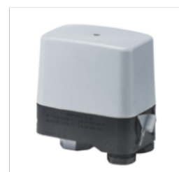
DANFOSS presostato cs 2-6 bar, dif. min. 0,72..1,0, dif.max. 1,0..2,0 ip55 g1/2" 031E021566
