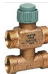
Valvula fancoil 3 vias con by pass HONEYWELL V5823C4013 Cuerpo laton, rosca 3/4" macho.PN16. kvs 2,5
