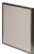
Filtro de aire MUNDOFAN MINIFIL ePM1 80% F9 500x625x48mm
